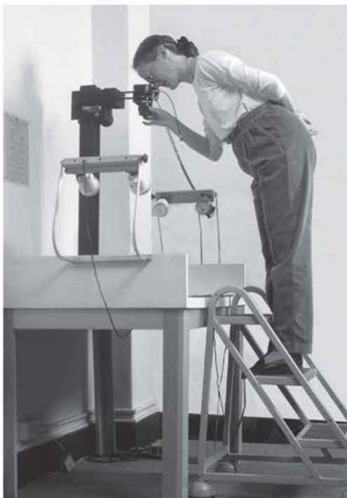
Figure 13: Using a ladder for focusing on large originals.
