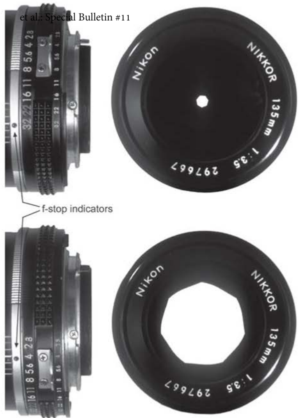
Figure 9: The top lens is set to f32; the bottom lens is set to f4
