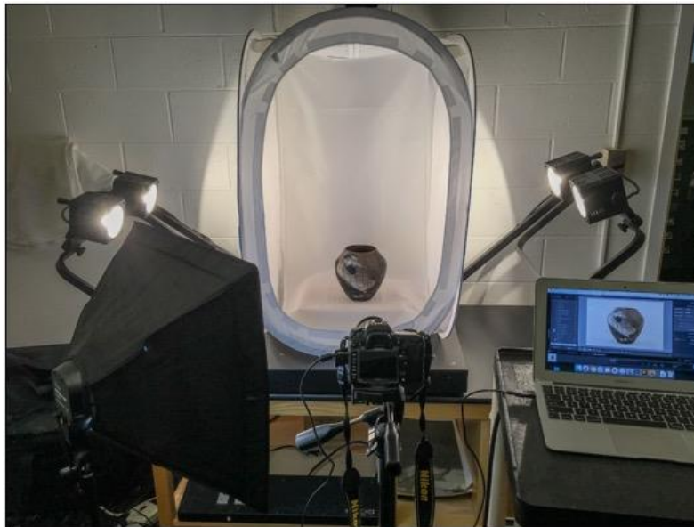
Figure 2: a typical photogrammetry set up includes a digital camera tethered to a computer and anchored to a tripod, lights, and a lighting tent (or other light-diffusing equipment). A Lazy Susan turntable (not pictured) is also recommended to gradually rotate the object as it is photographed.
