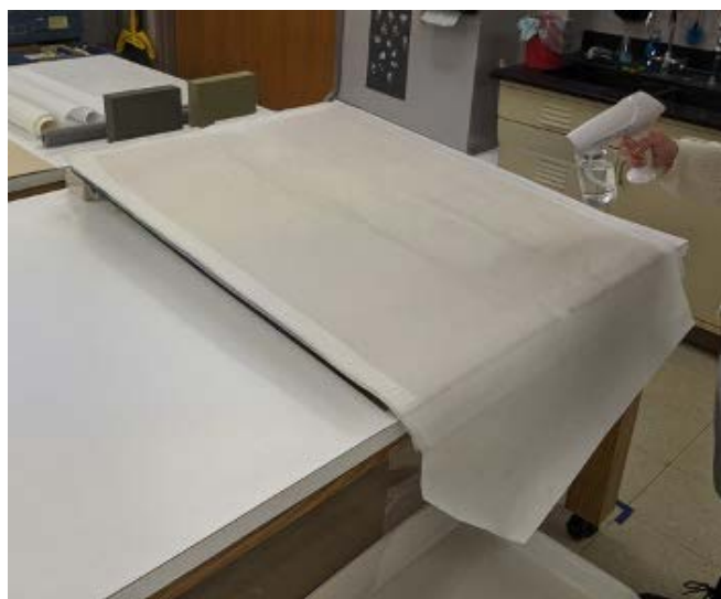
Figure 10: Washing with Nano Misting Device.
