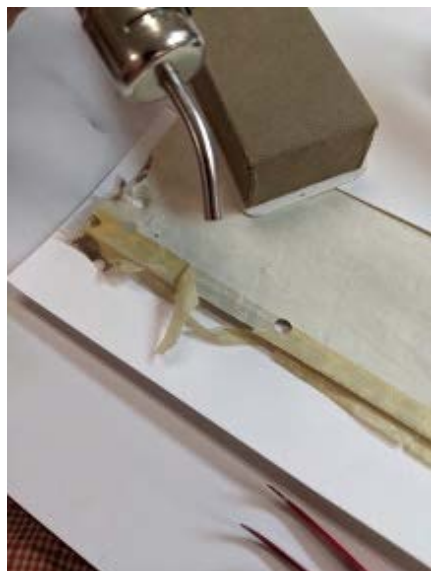
Figure 4: Softening tape with heat gun.
