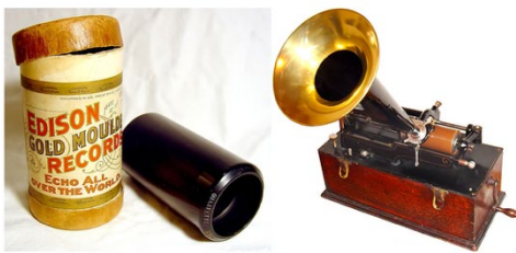
Figures 17, 18. Edison wax cylinder record and phonograph, both ca. 1905. Image source: The original uploader was Phonatic at English Wikipedia., CC BY-SA 3.0 via Wikimedia Commons.
