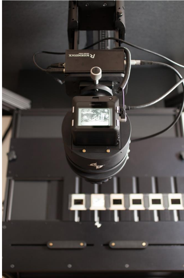
Figure 4 High-throughput capture of 35mm slides with DT RCam and Phase One IQ3 100MP digital back
